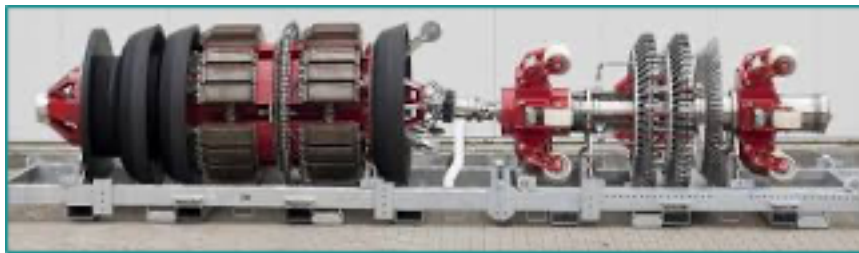
Figure 3-18: Intelligent pig
