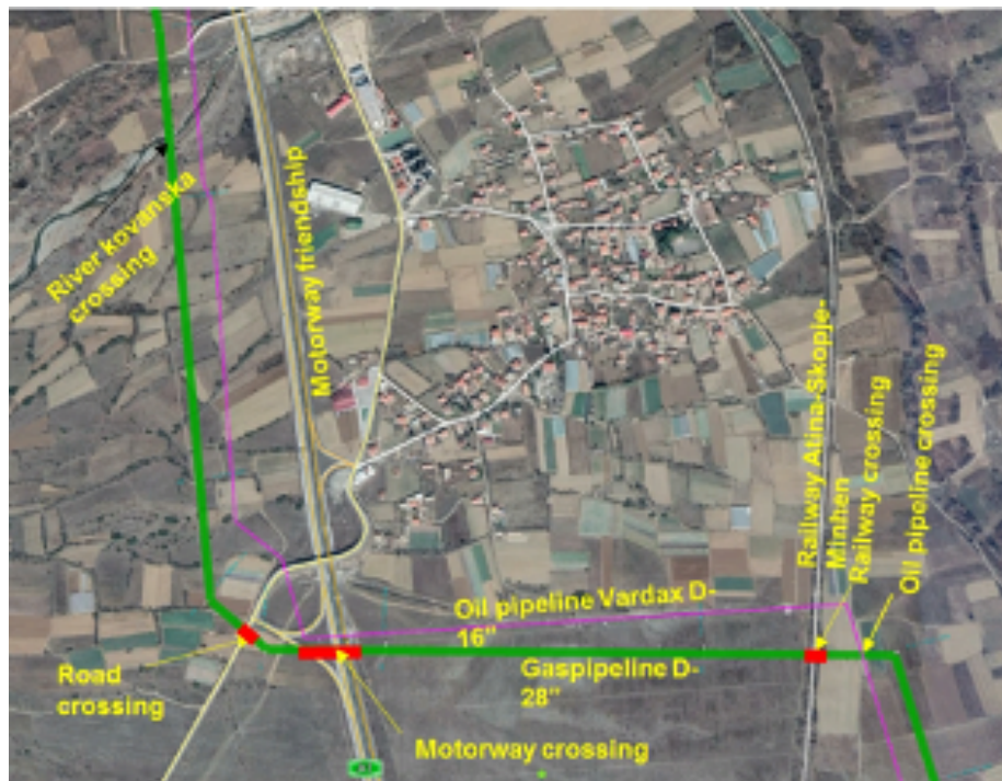
Figure 5-8: Passage under the oil pipeline at km 12+700, Railway line at km 12+755, Motorway A1 at km 13+600, Regional road at km 13+700 and Kovanska River at km 14+650
