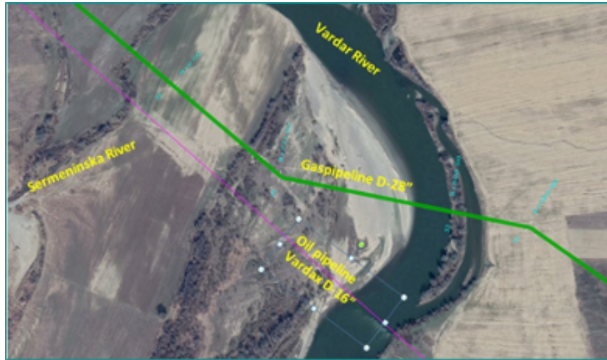
Figure 5-6: Crossing under the Vardar River km 8+500
