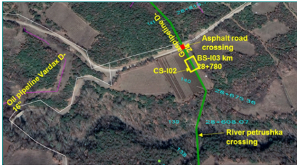
Figure 5-9: Crossing under asphalt road at km 28+780, BS-I03 at km 28+730, Cathodic Protection Station CS-I02 and passage under Petrushka River at km 28+600
